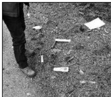
Fig. 1: CO 2 concentration measurement (in the foreground) and humidity of the soil profile (in the background)
