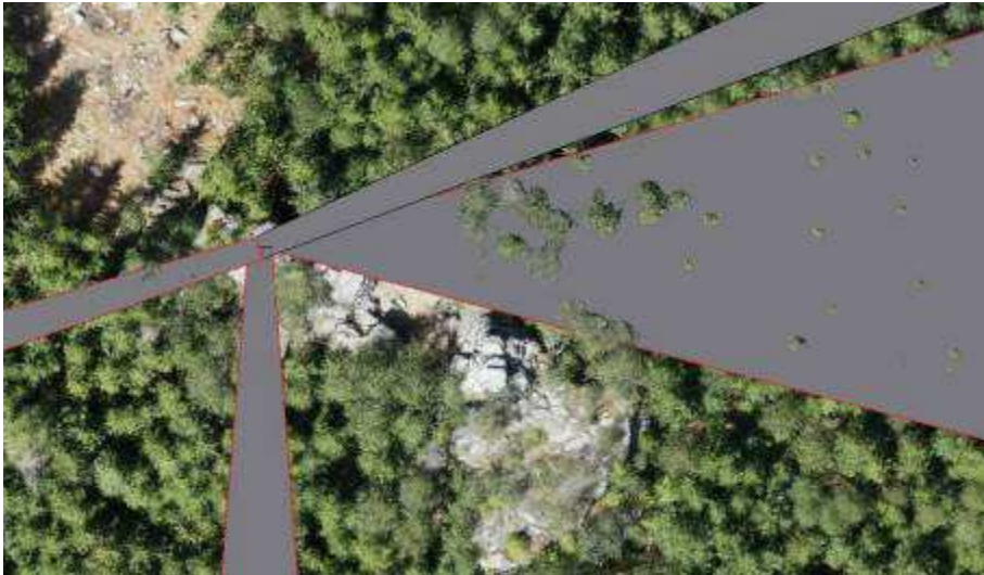
Fig. 4: Detail of intersection between the surface of the view fields and the digital model of the surface
