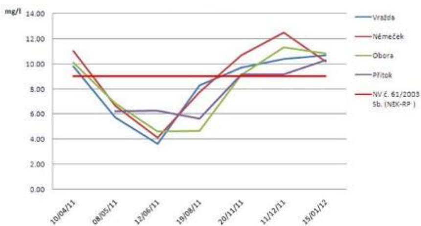
Fig. 4: Concentration of dissolved oxygen measured by a mobile multimeter
