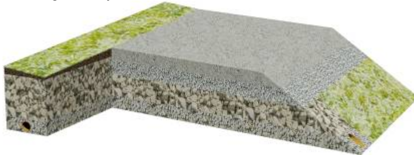
Fig. 2: Longitudinal and transverse drain (AutoCAD Civil 3D 2012).
